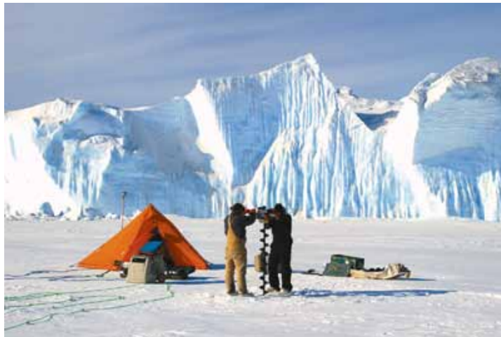
Figure 7: Deployment from a field camp. The entire SCINI ROV setup weighs less than 350 kg and was person-hauled by three or more people, in two sledges. A small tent was used for the control room.
