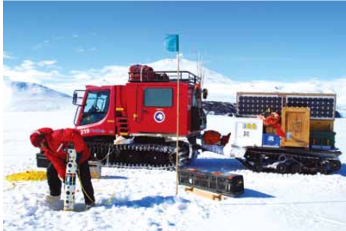
Figure 6: Deployment from McMurdo station. Up to six people and all equipment were transported in a tracked vehicle to sites within driving distance from the station. The cabin of the vehicle was used as the control room. Thanks to SCINI's small size and light weight, one person can easily launch the vehicle.
