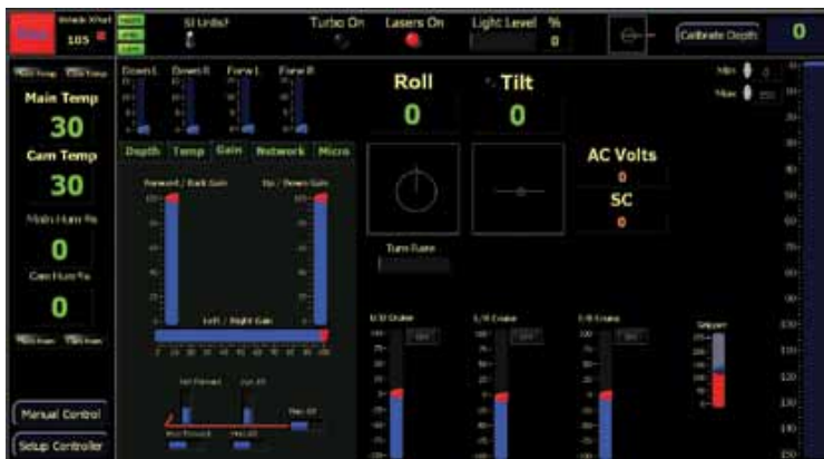
Figure 4: PCPilot software interface. This interface allows the pilot to monitor vehicle attitude and depth, housing temperature and humidity, and to control the lights, laser, and thruster gains.
