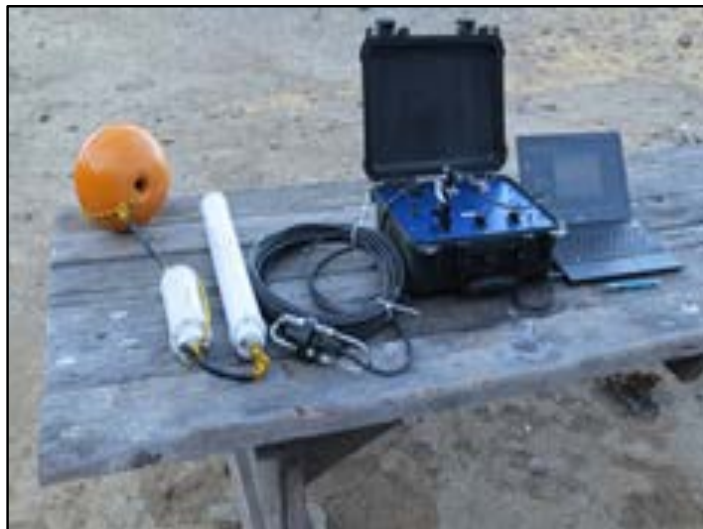
Figure 1: microMARS (left) attached to orange float (above it) and ARC-1 acoustic release device (right of it). Transducer and over-the-side cable (middle) is connected to a surface communication box and a netbook computer to run release device communication software.
