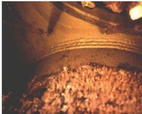
A weld inspection shows metal pitting
