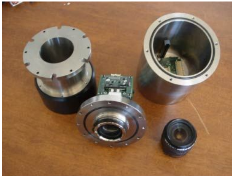
Modular Design: All SharkEye™ Cameras have Exchangeable Lens Systems (C-Mount or Canon EF), Internal CF FLASH Storage Cards and both Firewire and RS-485 Data Interfaces.
