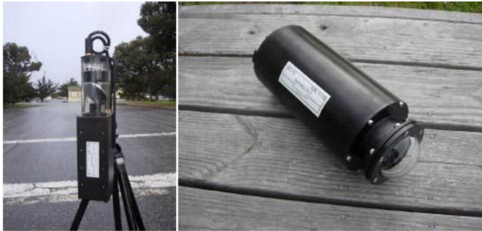
Custom Housings: With 360° rotating mirror (left), with dome port (right)
