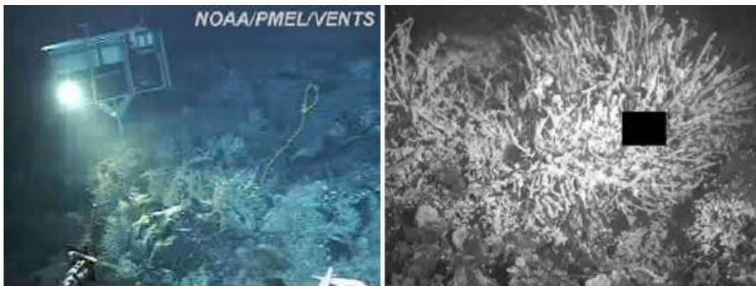
NOAA's NEMOnet autonomous observatory (left), and SharkEye™ picture of a tube worm colony with missing tile transmitted via an acoustic and a GEOS satellite link (right)
