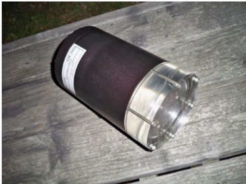
SL-3 Strobe (4000m depth rated version)
