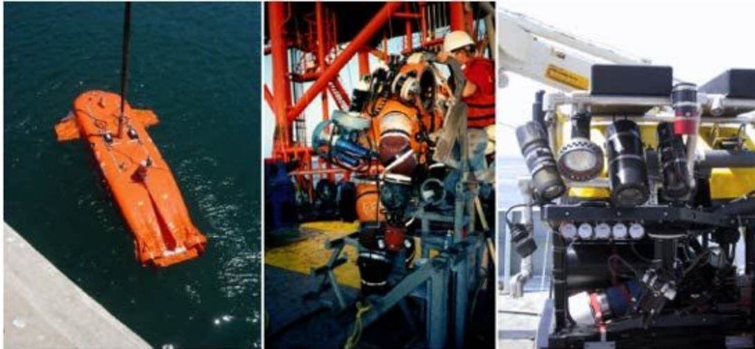
Dual SharkEye™ cameras on an AUV (left), single atmosphere diving suit (center), ROV (right)
