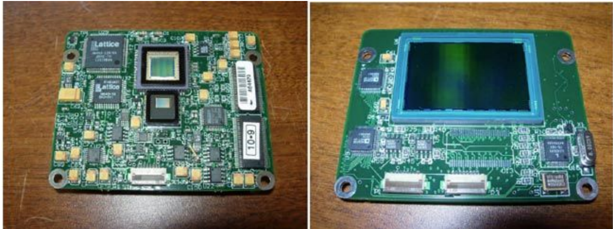
FISM-1 dual sensor module incl. very low light Electron Multiplier CCD (left). FISM-2 14-Megapixel CMOS sensor module (right)
