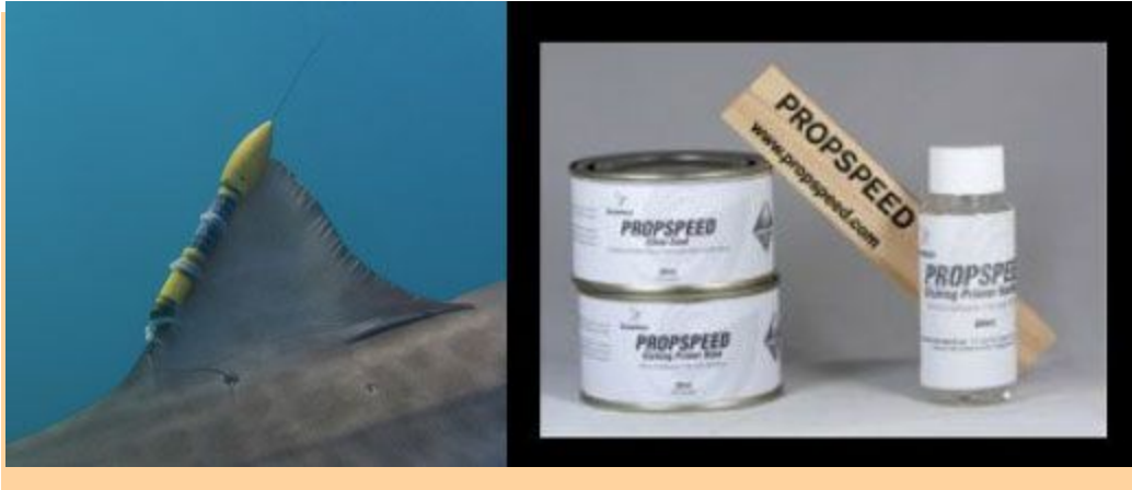
Figure 8.1 (right) shows a Propspeed coated tag in action and (right) Propspeed antifoulant paint kit.
