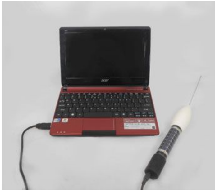
Figure 3.1 shows the set up between the MOD docking station and PC.
