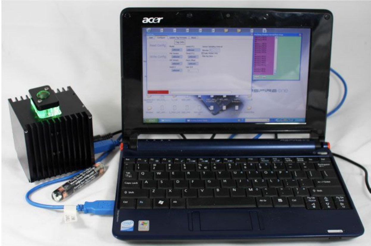
Figure 2: SeaTag-LOG™ system setup with ST-DOCK docking station connected to a small netbook PC via a USB cable. The SeaTag™ application for Windows is used to configure the tag and retrieve data logs.
