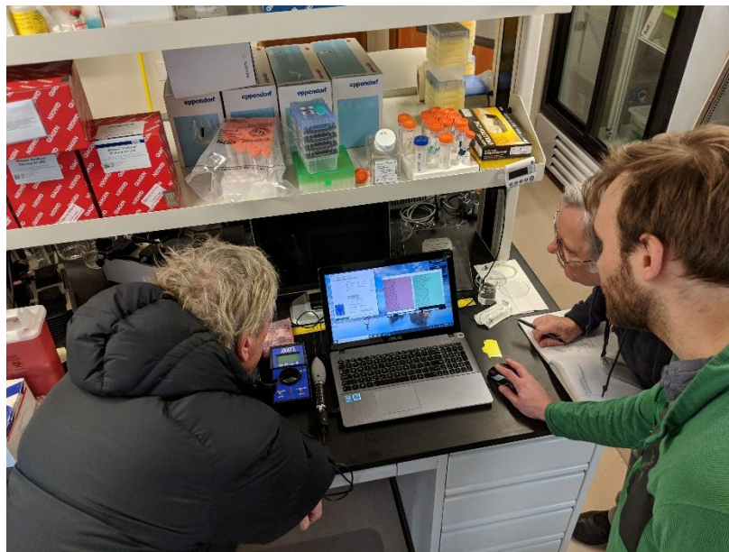
Figure 3: Rick Goetz (left), Andy Jasonowicz (center) and a third team member study the data return from the overnight fish test. Notice the tag to the left of the computer is linked to a docking station to recover a detailed report. To the left of the tag is the Pinger Dish from ATS (the blue box), which is used to activate the company’s JSATS pinger and set the Ping Repeat Interval (PRI) which determines the battery life of the pinger.
