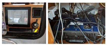
Installation on F/V Andree-Dean. The control display is installed in a console at the steering position. The STM-3 deck box is inside the
