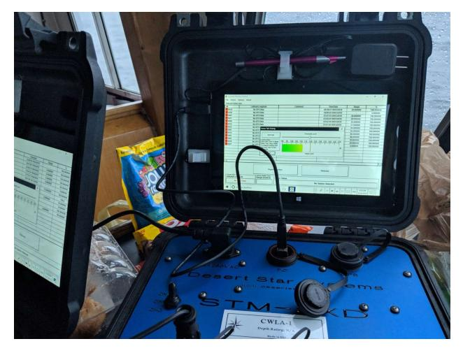
The DB-Control software is custom made to operate and release ARC units. This software is provided on a tablet, laptop or computer and is not free use. This software has several functions from noise testing to ensure there is no interference with other onboard gear, to interrogating releases and so on. For more information, view page 29 of this document.
