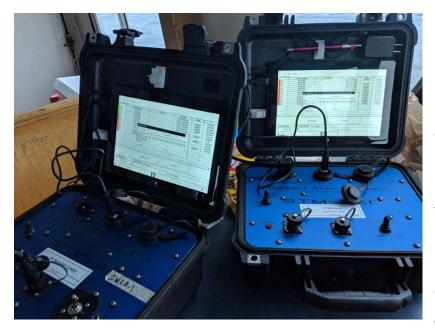
STM-3/4 (Signal converter for communication) The STM-3 deck box contains the sonar electronics that ranges to and commands the ARC-1XD acoustic releases. The STM-3 is mounted in a
