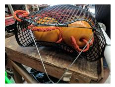
Not enough rope in bag: The mesh is folding over the floats, and the plastic may 'set' in this configuration after a prolonged time in cold water. If the current is high and the bag is 'leaning over', the floats may not exit the bag. Lesson: Fill each bag with enough rope to keep the floats unobstructed at the top. Be sure to tamp down the rope during the fill process such as with a broom. The rope lay needs to be tight in the bag.
