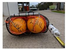
Enough rope in bag: The floats are near the top of the bag, and the mesh isn't folding over the float. These floats can be expected to exit the bag even when the bag is swept near horizontal in strong currents.
