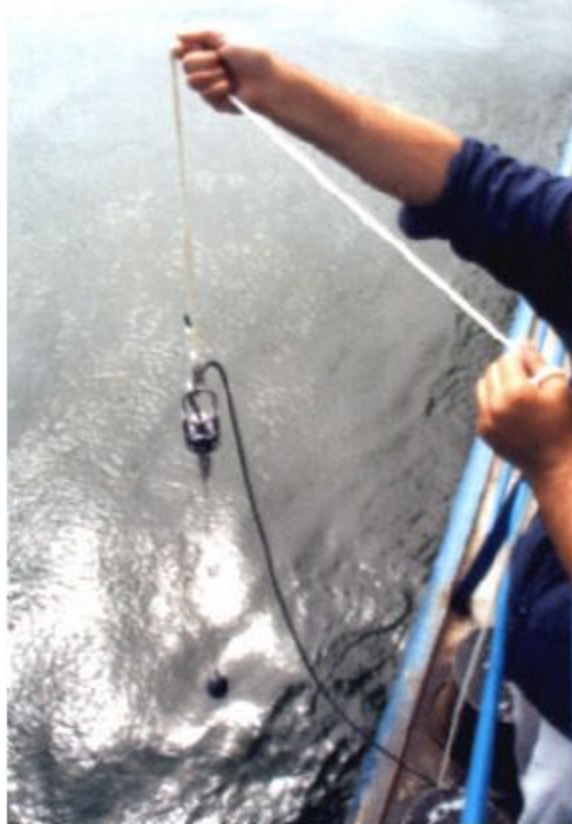
Figure 5.2: A Sonar Transducer Is Lowered Over The Side Of The Surface Vessel
