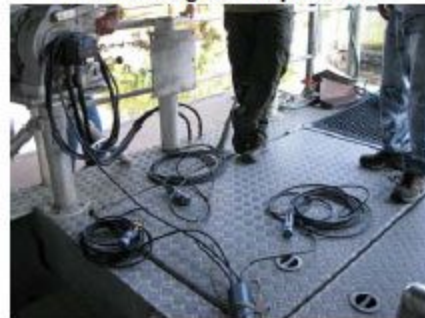
All responders connected with strain relief for each cable
