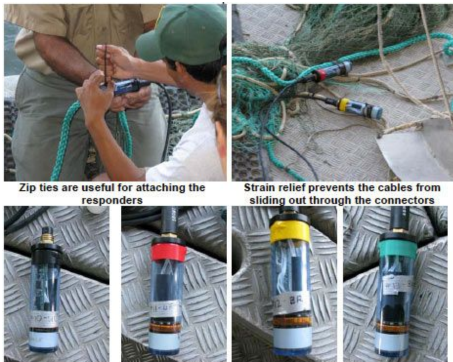
Figure 6: Attaching and Color Coding Responders
