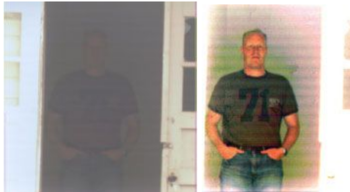
Motion blur control with AUTO Gain: 1/64 sec exposure (left) and 1/1500 sec exposure (right)
