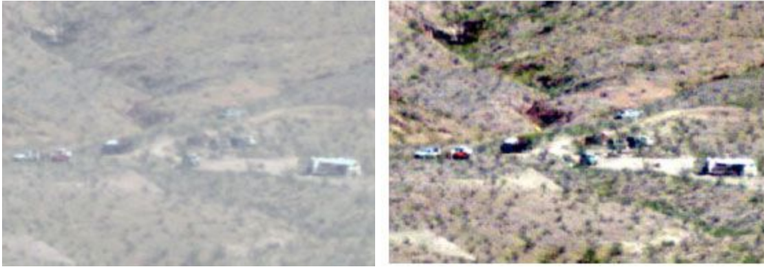
Contrast Enhancement with AUTO Gain: GAIN=x1 (left) and GAIN=AUTO (right)
