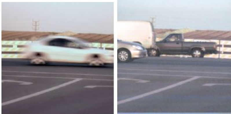
Motion blur control with AUTO Gain: 1/64 sec exposure (left) and 1/1500 sec exposure (right)
