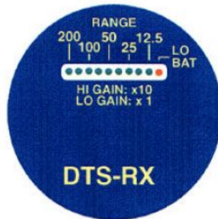
The LED strip Indicates Direction and Distance of the Transmitter
