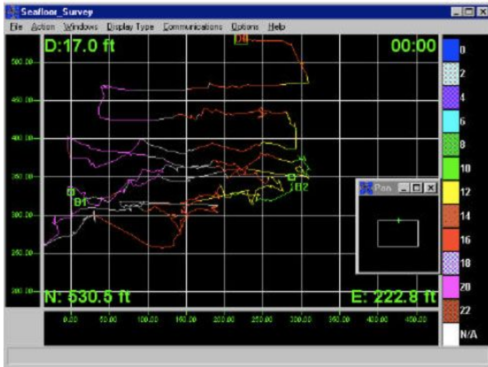
View of a Dive Site Generated By the DiveTracker™ DTX System
