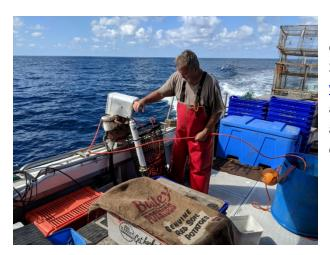
An Alstain Sheetmetal snood hauler (line hauler) employed to refill a release bag. The fill speed is 200 fathoms in 30 seconds. Click this link for a video of the release bag fill operation. Note that a random rope lay is used. Rope coiling is not advised as it puts tension in the rope and may cause snags.
