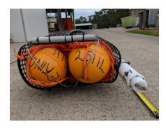
Enough rope in bag: The floats are near the top of the bag, and the mesh isn't folding over the float. These floats can be expected to exit the bag even when the bag is swept near horizontal in strong currents.
