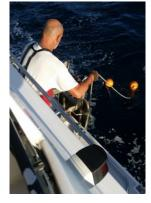
High visibility pop-up buoys: High visibility buoys are another important consideration to minimize gear loss. 8" (20cm) diameter orange hard floats (depth floats) float almost entirely above the waterline and are thus visible from a long distance. Select a color that clearly stands out against the background and allows the pop-up buoys to be spotted quickly after pop-up.
