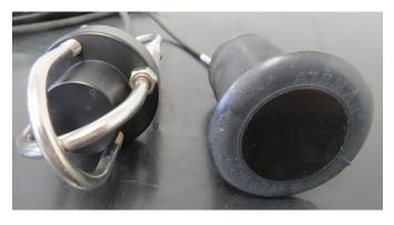
The over-the-side transducer (left) and the through-hull transducer (right). The through-hull transducer allows ranging to and commanding the ARC-1XD releases while your boat is underway. The over-the-side transducer has limited such capability when lowered over the side and weighted. But it should only be used as a last resort.
