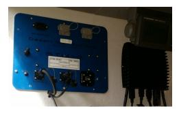
Permanent installation of the STM-3 deck box (F/V Seeking): The STM-3 instrument panel is removed from the Pelican case and mounted on a bulkhead of the boat (left). The through-hull and the over-the-side sonar transducers are wired to the box and selectable via a toggle switch. An industrial PC (black box on right) runs the DB-ARC control software.
