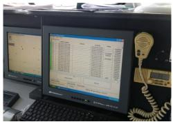
The ARC-1XD releases are controlled via the control screen and keyboard mounted in the wheel house.
