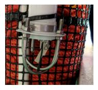
Snagged lever: The lever arm is pointing parallel to the bag, not away from the bag. This resulted in the release cord snagging the lever arm, preventing it from fully opening and releasing the release cord. Lesson: Make sure the ARC-1XD is mounted to the bag such that the tip of the lever arm points away from the bag.
