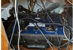
Installation on F/V Andree-Dean. The control display is installed in a console at the steering position. The STM-3 deck box is inside the console and remains mounted in its Pelican case for easy swap-out.
