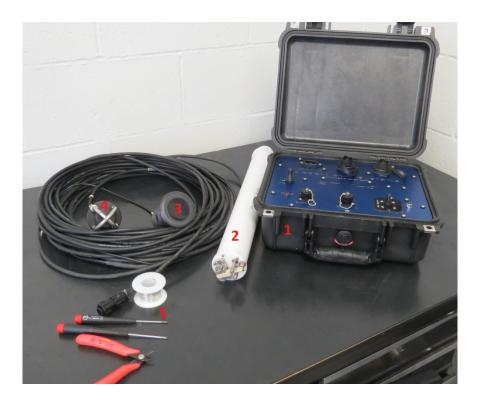
The Desert Star Systems provided components for a ropeless fishing system including (1) the STM-3 deck box for remote control, (2) the ARC-1XD acoustic release, (3) the through-hull transducer to range to and command the ARC-1XD while underway, (4) an 'over the side' transducer for various test functions and as backup, (5) a set of small tools and supplies to re-arm and service the ARC-1XD.
