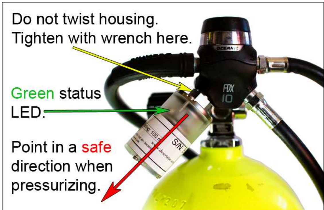
Figure 2: Pressure transmitter (APA-TX) mounted on one of two high-pressure ports on a SCUBA regulator first stage. A SPG must be mounted on the second port. Tighten with 3/4" wrench (never tighten by turning the housing), and point in safe direction during pressurization in case of pressure sensor fail leading to housing pressurization.
