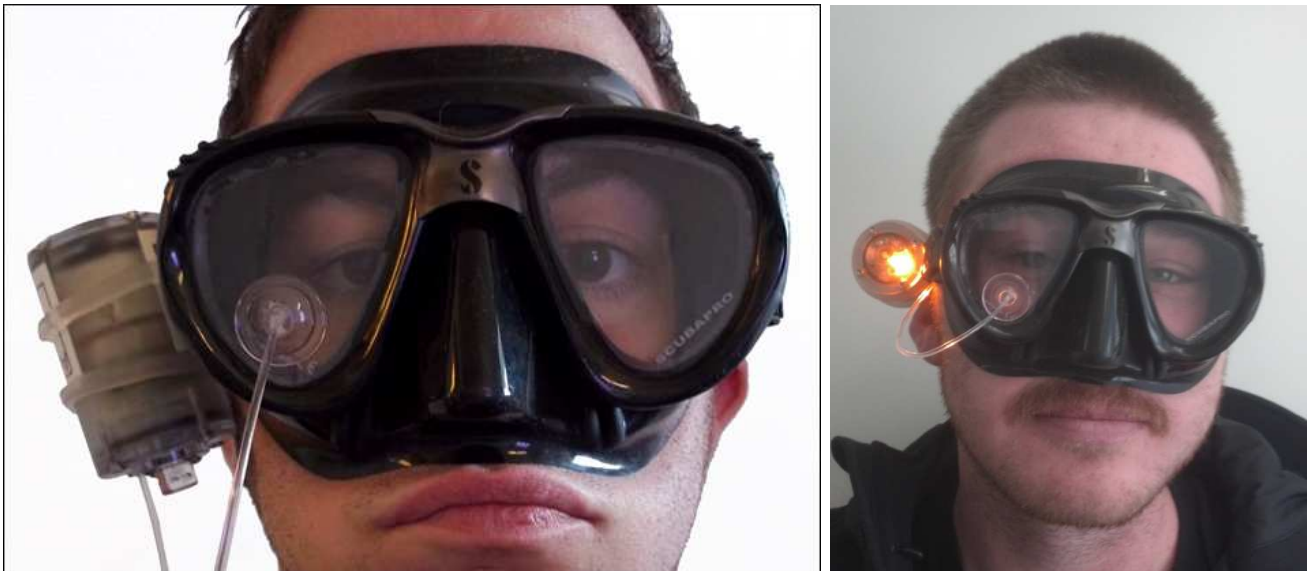
Figure 3: Alert unit in vertical and horizontal mounting configuration. Horizontal has reduced snag potential and provides maximum LED visibility when facing a buddy. Vertical provides a better sonar beam pattern for buddy communication and LED visibility from behind.
