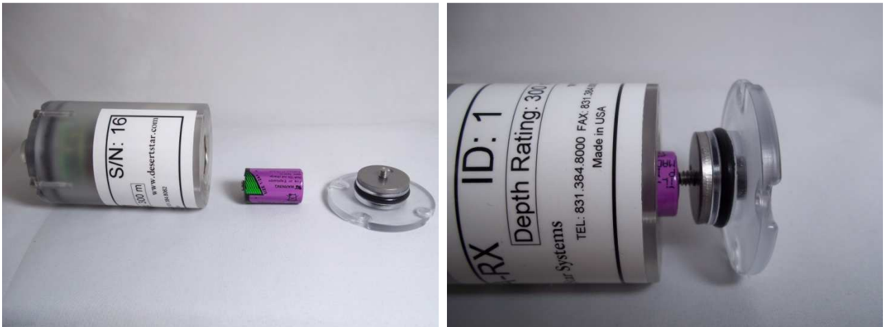
Figure 5: Battery alignment for insertion. Positive terminal goes in first.
